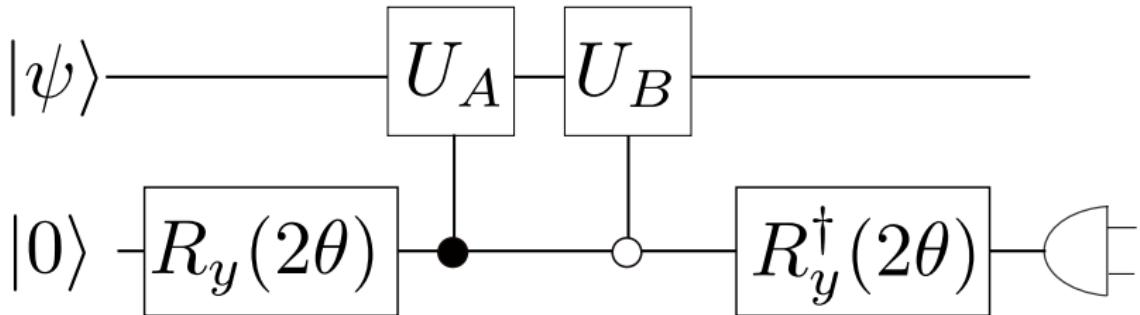
$$\begin{aligned} |\psi\rangle |0\rangle &\rightarrow |\psi\rangle (\cos \theta |0\rangle + \sin \theta |1\rangle) \\ &\rightarrow \cos \theta |\psi\rangle |0\rangle + \sin \theta U_A |\psi\rangle |1\rangle \\ &\rightarrow \cos \theta U_B |\psi\rangle |0\rangle + \sin \theta U_A |\psi\rangle |1\rangle \\ &\rightarrow (\cos^2 \theta U_B + \sin^2 \theta U_A) |\psi\rangle |0\rangle \\ &+ \sin \theta \cos \theta (U_A - U_B) |\psi\rangle |1\rangle . \end{aligned}$$
